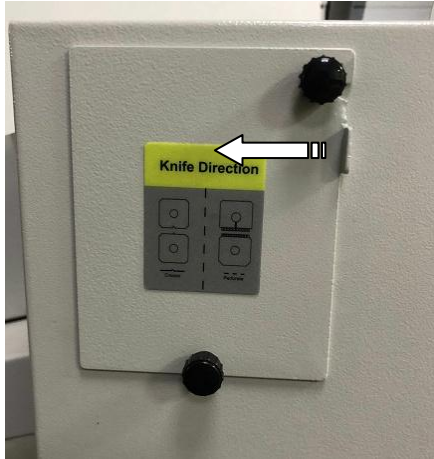
Step 1: Loosen the 2 screws on the blade gate and turn the blade to left to open it.
