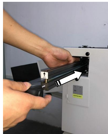
Step 3 :Push the blade all the way into the machine.
