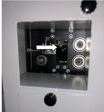
Step 1: Loosen the 2 screws on the blade gate and turn the blade to left to open it.
