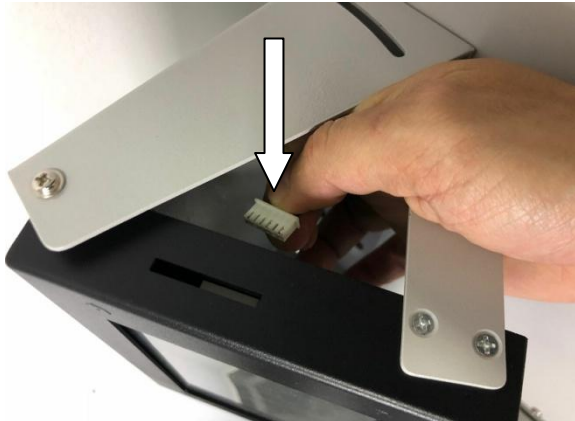
Step 3: Plug the cable to the touchpad.
