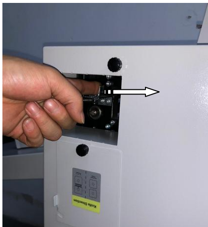
Step 2: Push the lever of the blade lock to right.
